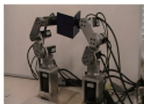
Fig.2 Reconfigurable Robot System
