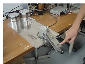
Fig. 3 Stiffness Adjustable Tendon
