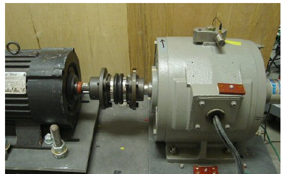
Fig. 1. Vibration suppression control using acceleration sensor.
