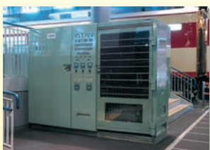
ざせきせやくしすてむ 座席予約システム: マルス1/みどりの窓口の先がけ MARS1/JR Reservation Ticket Offices "Midori-no-madoguchi" Magnetic electronic seat reservation system
